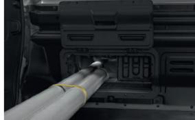
Bulkhead flap lifts to allow extra long objects – up to 3.75M in the L1 Primastar or 4.15M in the L2 Primastar.\*
